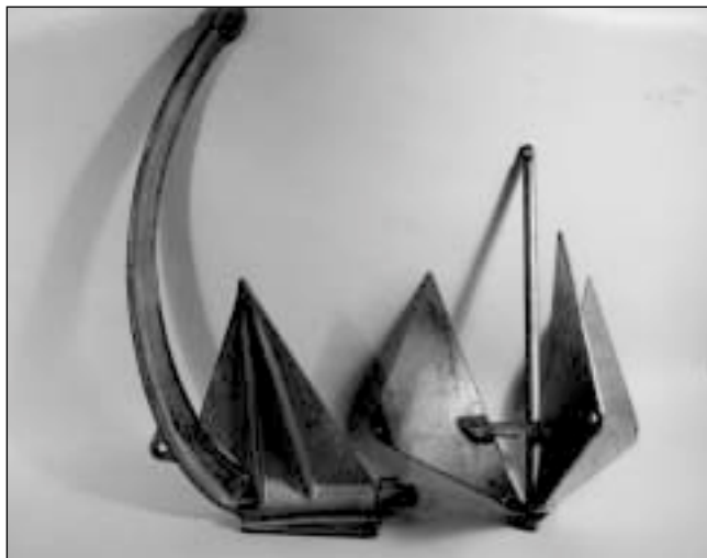
Left: The Barnacle, shown at the left, is an unusual one-fluke anchor that stows flat. At the right is the Bulwagga anchor that challenges the Spade in every category. The Bulwagga's only shortcoming: It's clumsy to handle and difficult to stow.
