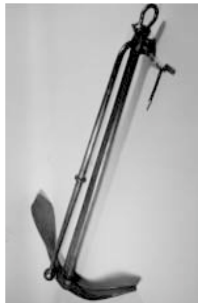
Left: This 1914 Herreshoff design, once the world's most popular anchor, has been out-done by more modern anchor but is still favored as a 'rock' anchor. This Herreshoff, which retails for $375, sets quickly. It did well in this reset test. Its weakness is holding power. Above: The Herreshoff folds for stowage. There is a smaller size whose threaded shank makes an even smaller package to stow.
