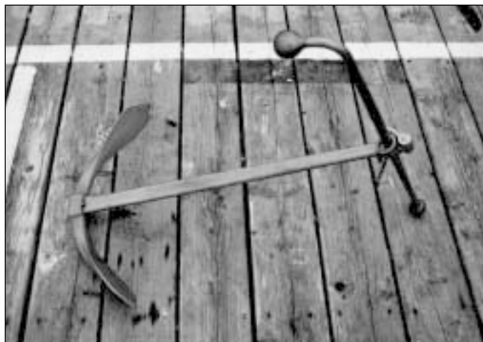
Left: This 1914 Herreshoff design, once the world's most popular anchor, has been out-done by more modern anchor but is still favored as a 'rock' anchor. This Herreshoff, which retails for $375, sets quickly. It did well in this reset test. Its weakness is holding power. Above: The Herreshoff folds for stowage. There is a smaller size whose threaded shank makes an even smaller package to stow.
