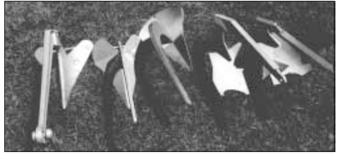
Above: Shown here are several 'old reliables,' plus the French-made Spade. From left to right are the CQR, Delta, Spade and two versions of the Supermax, one with a fixed shank, the other adjustable for different type bottoms.
